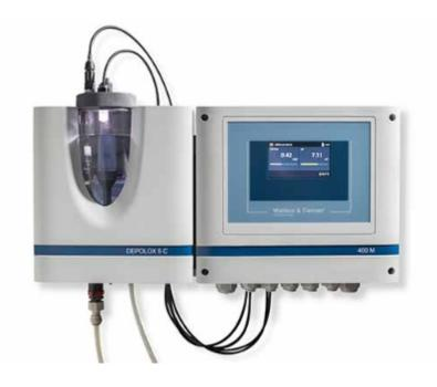
Do not power the unit until water flows trough the cell. Avoiding this will polarize electrodes and delay by up to 24 hours chlorine reading (static electricity will build up onto reading electrodes and negative reading will be displayed). Wire accordingly:
