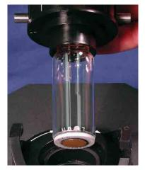
Patented Ultrasonic Autoclean System Keeps the optical chamber clean in finished or raw water applications.
