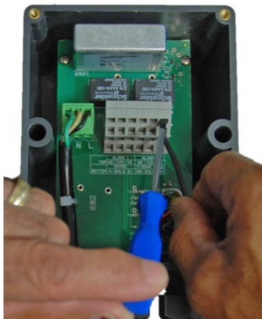
Figure 6: Electrical Connections on Terminal Block (P1)
