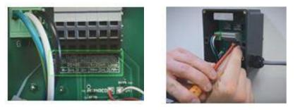
All electrical connections are made inside the junction box. Choose the appropriate cable gland for each connection.
