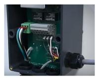
The MTOL+ has outputs for both 4-20mA and Modbus. These are located on grey terminal block on the lower row. The connections are marked on the PCB surface. These spring-loaded terminal blocks are operated by inserting a 3mm (1/8") flat blade screwdriver in the smaller opening directly above the connection. Tilting the screwdriver up will open the connection and allow for wire insertion.
