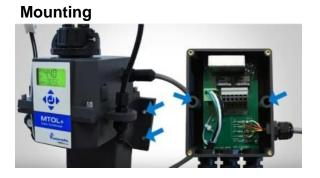
The junction box is located under the sensor portion as shown above. Use appropriate screws and hardware as needed for mounting the instrument to the chosen surface.
