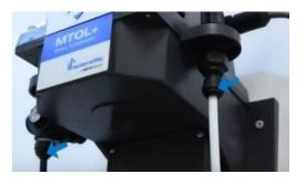
The lower sections of the sensor are equipped with push to connect fittings for use in both the intake and drain. Use ¼" OD tubing. Flexible polyethylene or polypropylene tubing is recommended. To lower algae growth opaque tubing is highly encouraged. Make sure the flow through is connected before starting the water flow. We recommended that the flow through be tested for leaks before inserting it into the sensor.
