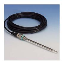
The UV lamps produce a considerable amount of heat, which is carried away by an adequate flow of water. If this flow of water is not ensured, overheating can occur, possibly resulting in damage to the UV disinfection unit. A Pt100 temperature sensor is installed in the UV disinfection unit on one of the lateral flanges for monitoring the water temperature. As soon as the set maximum water temperature is exceeded, an alarm signal is given and the unit is switched off.
