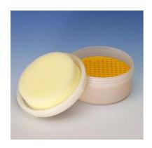
Mercury is toxic and must be collected immediately if it is spilt. The mercury collector is a screw-top container made of polyethylene. The lid contains a special foam insert and the container a mercury separation sheet. (Optional; part number W3T164613)
