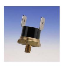
A bimetallic switch is fitted on the side flange to provide additional temperature monitoring. This switches the lamps off if the Pt100 temperature sensor fails and the surface temperature in the disinfection chamber, as measured on the lamp flange, rises above the maximum threshold, which is set at 65°C.
