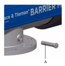
When the UV disinfection unit is exposed to increased corrosion, e. g. due to brine or salt water, the installation of a sacrificial anode, part No. W3T274659 is absolutely necessary as corrosion inhibitor. Sacrificial anodes are dissolving and must therefore be checked in regular intervals, depending on the application and the local conditions, and replaced if necessary.
