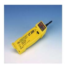
The lamp tester runs on a 9 V battery; it transmits a high-voltage pulse to the lamp. A brief flashing of the lamp indicates it is functional. (Optional; part number W2T507701)
